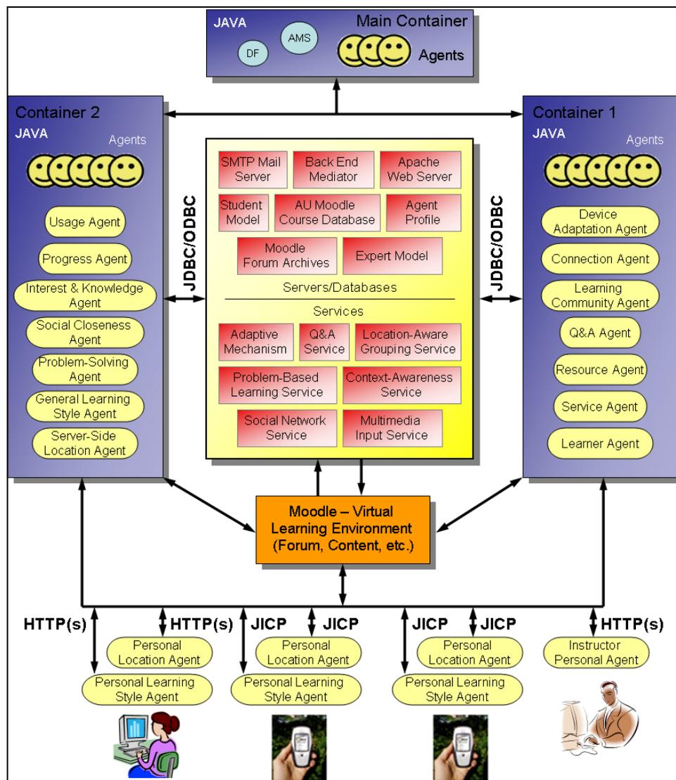
FIGURE 1. Architecture of the adaptive mobile learning environment.
